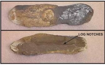
STEP 2. LOG #1 (SRV2065-704) Place log #1 on left flat side of the burner assembly. Pull the log and slide it to the right until the notches under the log are in the burner grooves.
